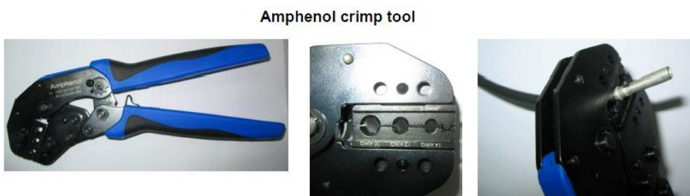
Figure 4-18 wire end crimping method
